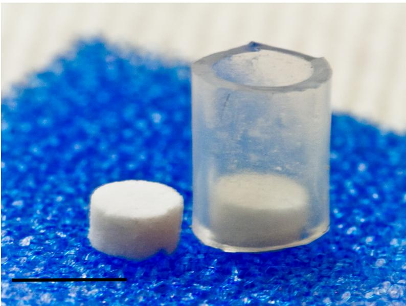
Fig. 2. Calcium polyphosphate (CPP) disc enclosed by silicone tube forming a culture well preventing cell leakage. Scale bar indicate 5 mm.
