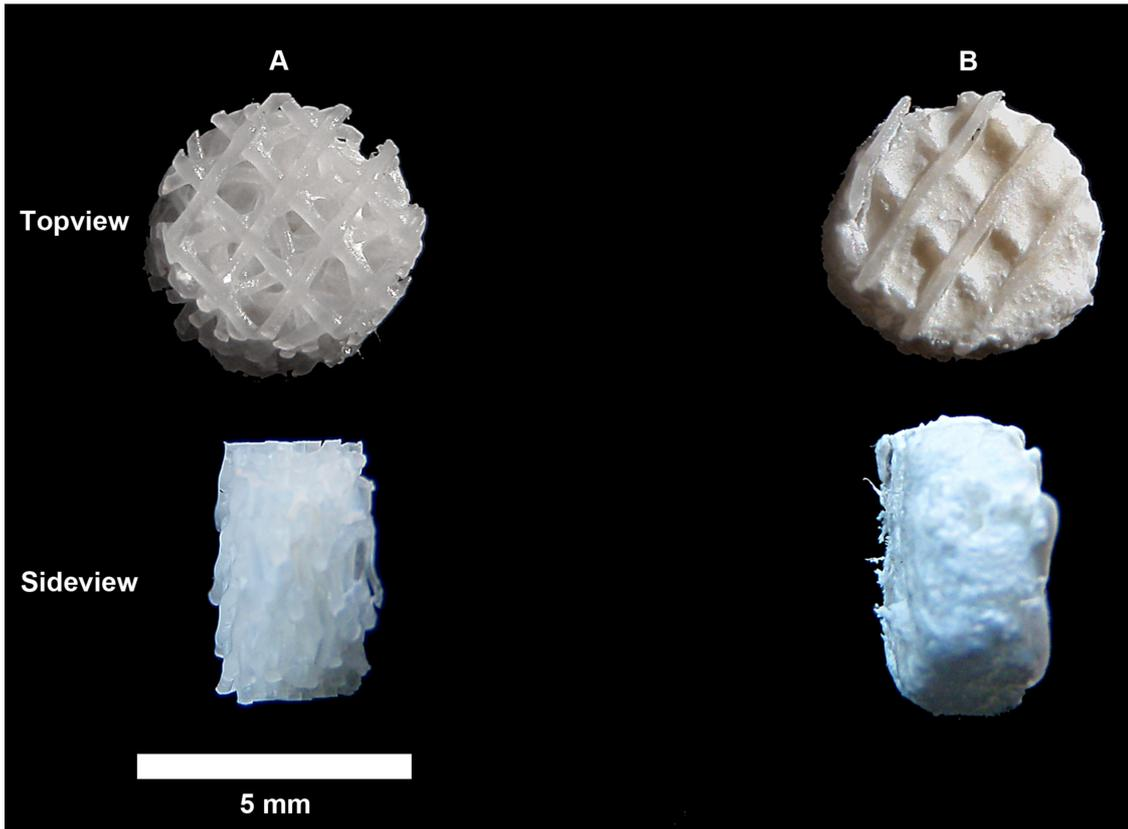
Figure 9 Macroscopic pictures of (A) FDM scaffold. Note that the shift in fibre orientation of  $105^\circ$  between layers creates the grid-shaped scaffold structure. (B) SGS made by combined FDM and TIPS-FD. Scale bar indicates 5 mm.
