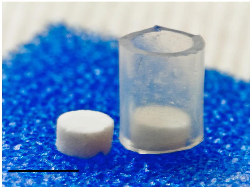
Figure 13 CPP disc enclosed by silicone tube forming a culture well preventing cell leakage. Scale bar indicates 5 mm.
