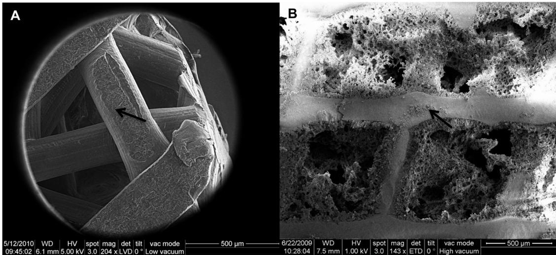
Figure 10 SEM images of (A) FDM scaffold. Note that the shift in fibre orientation of  $105^\circ$  between layers creates the grid-shaped scaffold structure. (B) SGS made by combined FDM and TIPS-FD. Note that TIPS of the solvent PCL creates micro-pores of 100-250  $\mu$ m within the larger macro-pores. (↗) Arrow indicates PCL fibre. Scale bar indicates 500  $\mu$ m.
