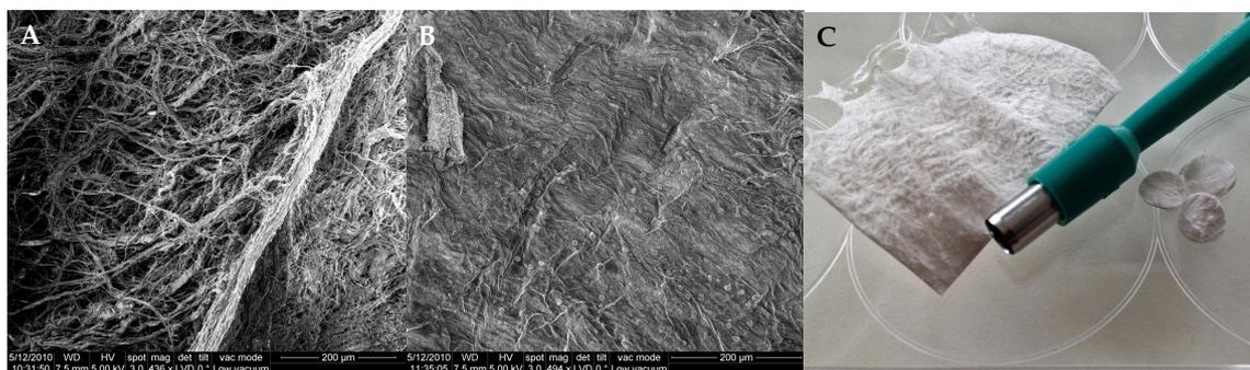
**Figure 7** SEM of the collagen type I/III scaffold. **A:** The porous side with 20-100- $\mu\text{m}$  large pores. This part of the scaffold was seeded with AT-MSC. **B:** The compact side of the scaffolds ensured cell-entrapment. **C:** Skin biopsy punch for the cutting of scaffolds.
