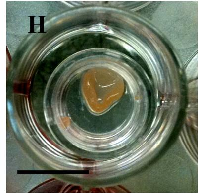
Fig. 3. Macroscopic tissue constructs multilineage progenitor cells (MLPC) cultures after five days (A-E) and 14 days (F-H). Row 1 and 2 represent biological replicas of A-E cultures. MLPCs cultured on calcium polyphosphate (A, F), non-coated membrane inserts (B, G), collagen I coated membrane inserts (C), collagen II coated membrane inserts (D) and collagen IV coated membrane inserts (E, H). Scale bar indicate 10 mm.
