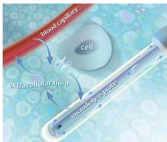
Figure 3. Schematic overview: Basic principle of microdialysis
