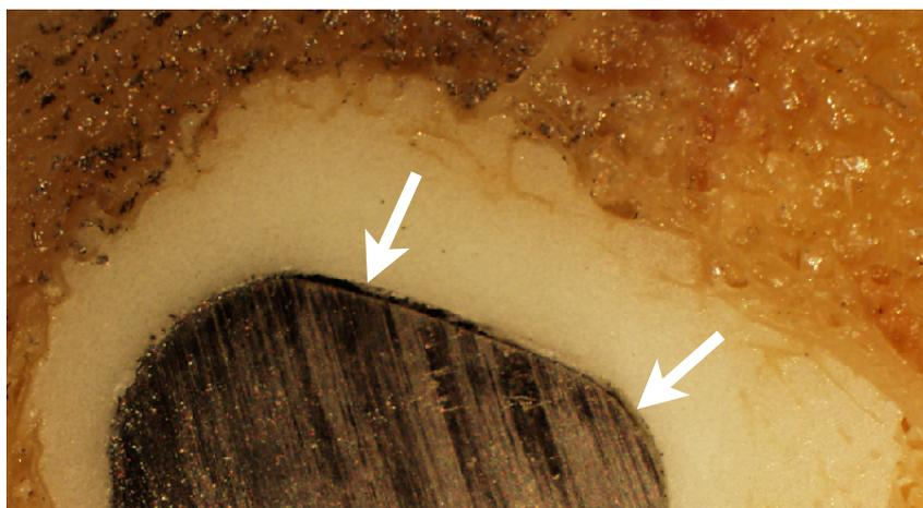
**Figure 2.** Example of separation between prosthesis and cement (block arrows); image is taken from Study II, but in clinical situation it would represent debonding.
