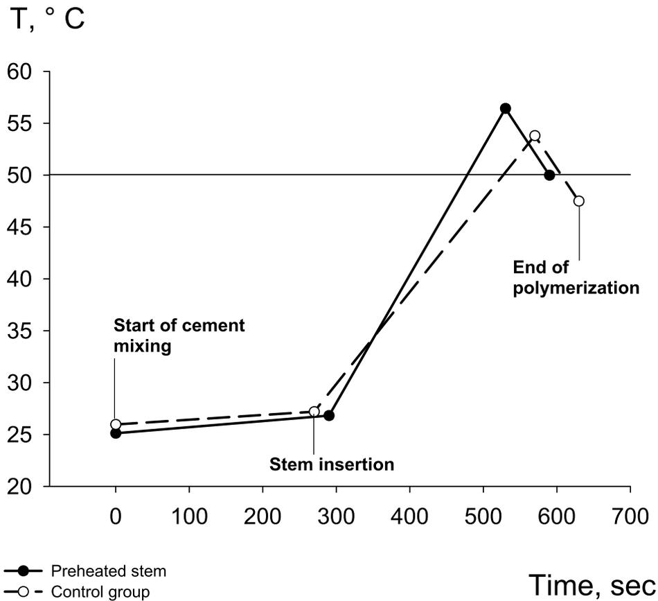
**Figure 20.** The mean of the bone–cement interface temperatures obtained during cementation of 33 preheated and 30 non–preheated femoral components in THA. The time points at cement mixing, stem insertion, peak temperature and the end of cement polymerization are marked with circular symbols.
