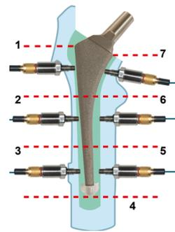
**Figure 15.** Peak pressure recordings during stem insertion. Measurements at the medial and the lateral zones at the same level belong to the same region.
