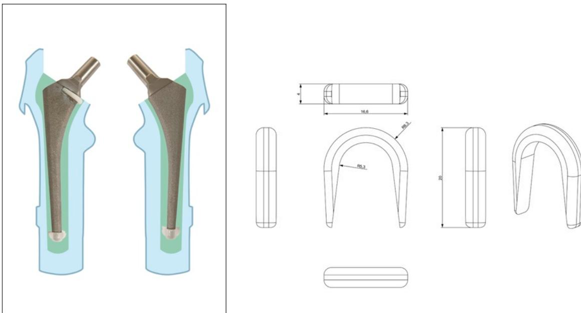
**Figure 4.** Femoral components. A proximal centralizer on the left stem and distal centralizers on both stems. Design of the custom-made proximal stem centralizer.
