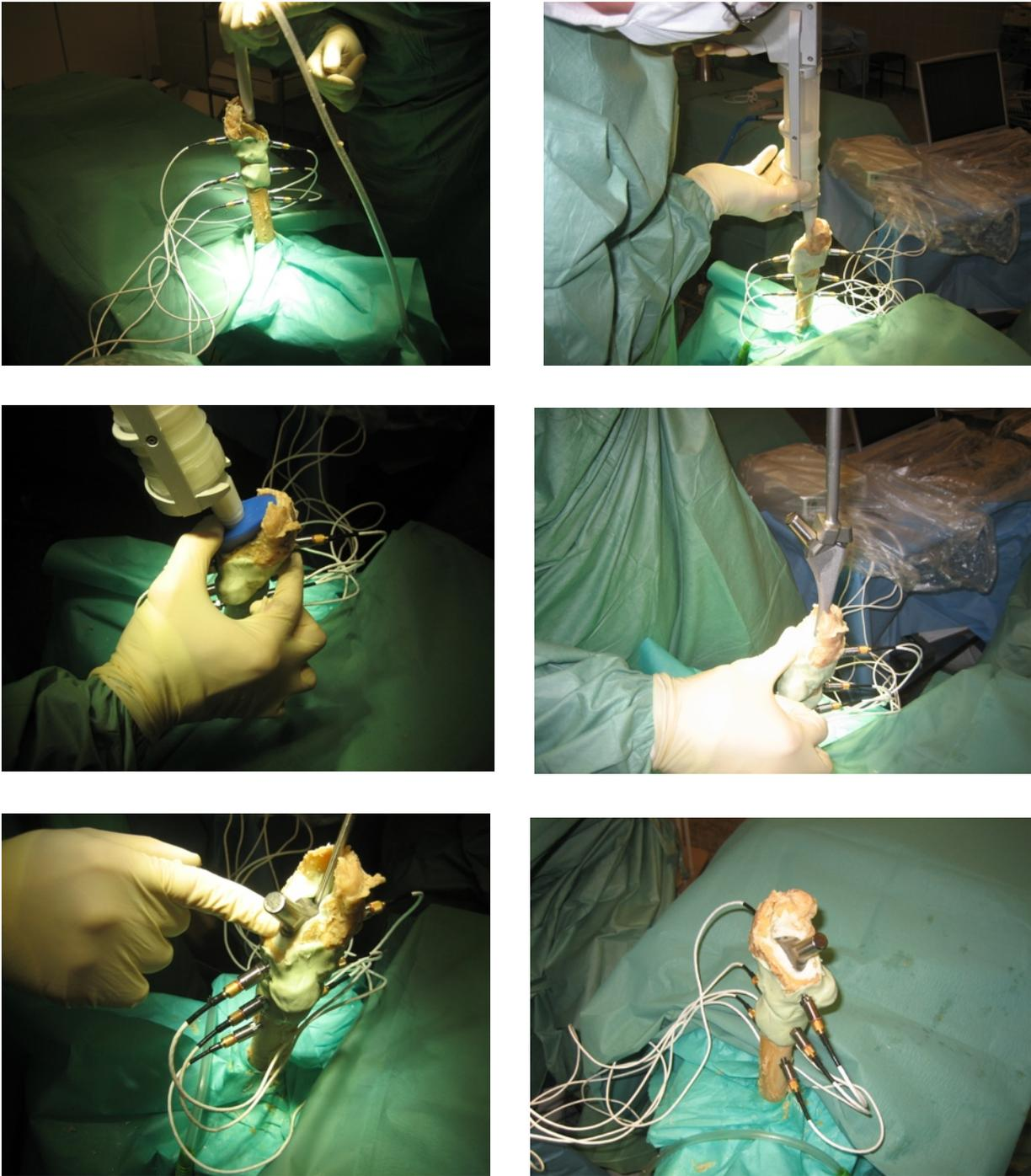
**Figure 5.** Stepwise preparation of femoral canal and stem cementation, from top-left to right-bottom: Lavage of medullary cavity, retrograde cement application, pressurizing, stem insertion and finally implant in situ. Six pressure transducers on medial and lateral side could be seen.
