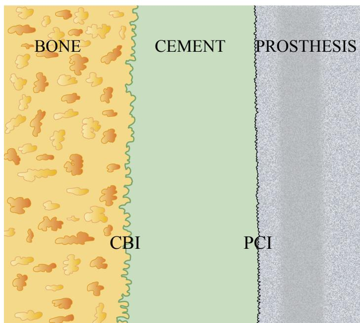
**Figure 1.** Prosthesis–cement–bone composite with two critical interfaces: prosthesis–cement interface (PCI) and cement–bone interface (CBI)
