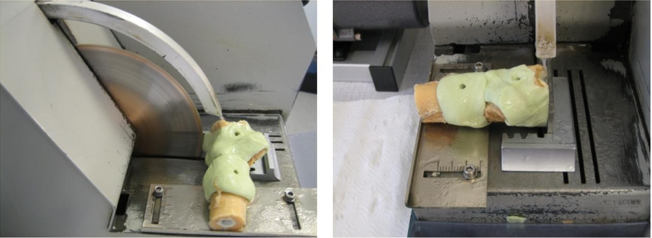
**Figure 8.** Sectioning of cemented implant–bone specimens.
