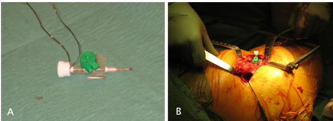
**Figure 13 A-B.** Temperature measurement at cement-bone interface. A probe with two thermocouples before application (A) and during the surgery (B).
