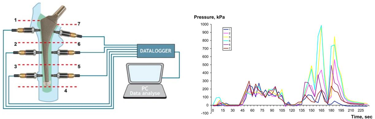
**Figure 6.** Schematic cartoon of the positions of the pressure transducers and pressure recorder. On the right a typical pressure profile during cementation is shown. Small pressure elevations in the beginning of curves correspond to cement application and pressurizing whereas large peaks are related to stem insertion.
