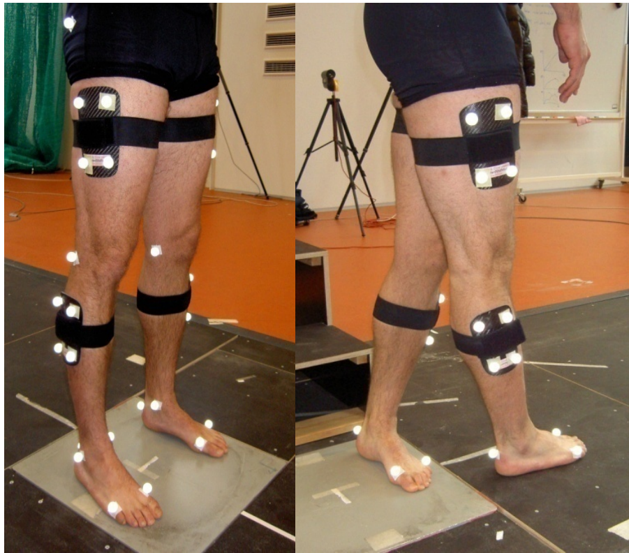
Fig 16: Left picture shows the marker model used for the static trial. Right picture shows the pivoting maneuver and the marker model used while performing the tasks 109, 110 .
