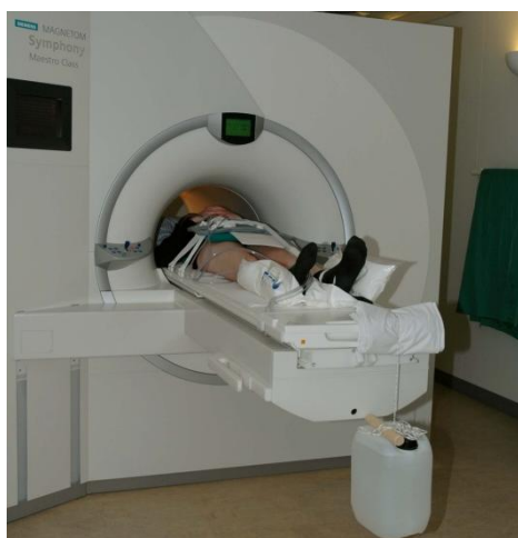
Figure 12. MRI and traction device that pulled the leg distally with a load of 10 kg.
