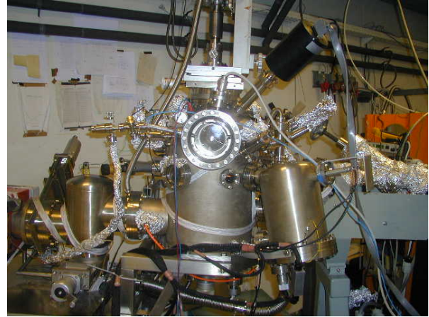
Fig. 3. XPS setup. The discs were placed in the Ultra High Vacuum chamber with a base pressure of approximately 10 -10 torr.
