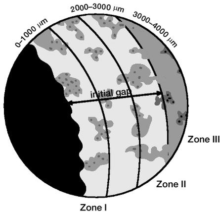
Figure 2. The volume fraction of new bone formation, grafting material and unmineralized tissue were quantified in two zones well defined from the implant surface: Zone 1: 0–1000  $\mu\text{m}$ , zone 2: 2000–3000  $\mu\text{m}$ . The volume fraction of bone was quantified in zone 3, 3000–4000  $\mu\text{m}$  from the implant surface.
